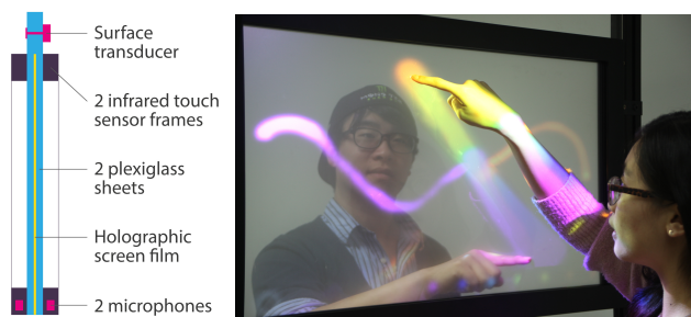
Figure 1. (a) Sectional view of TransWall and (b) users playing the game "Chromatic rubber band"
